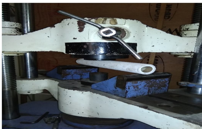
Fig 9 Experimental setup of Glass fibre roller
