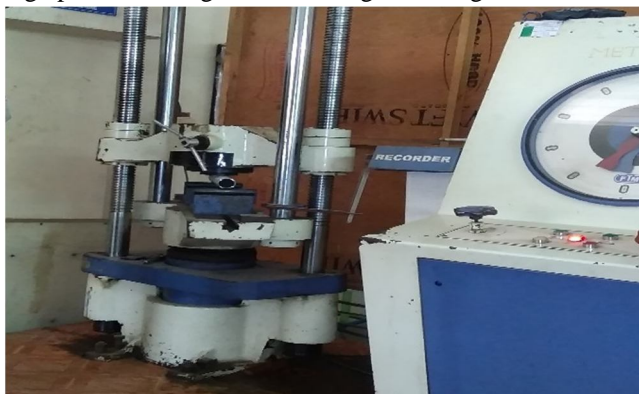
Fig. 8 Experimental setup of MS roller
