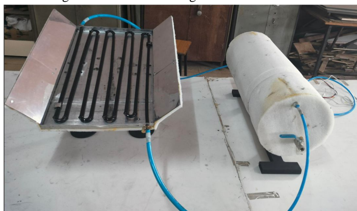
Figure 16 Final experimental setup of Solar water heater
