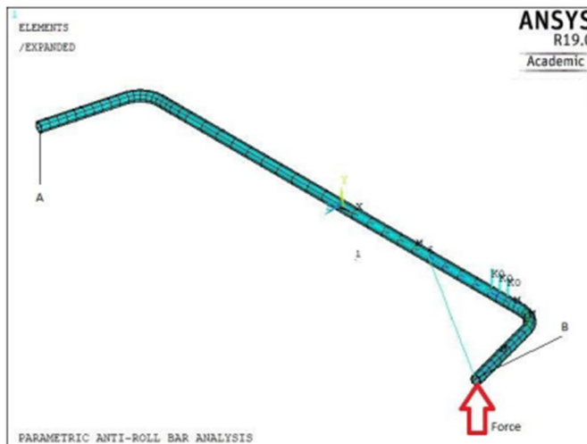
Figure.6.3 Geometric of Anti-roll bar in ANSYS APDL
