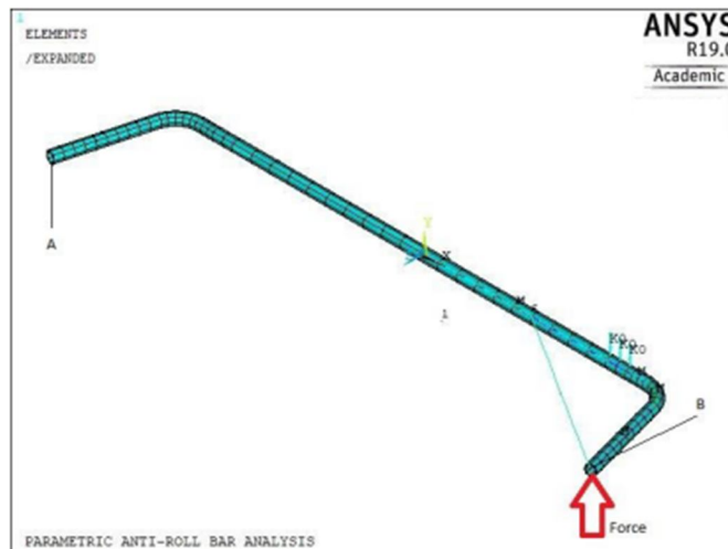
Figure.6.3 Geometric of Anti-roll bar in ANSYS APDL
