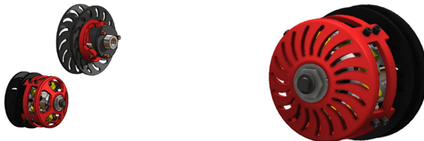
Fig 3.1 The assembly of CVT
