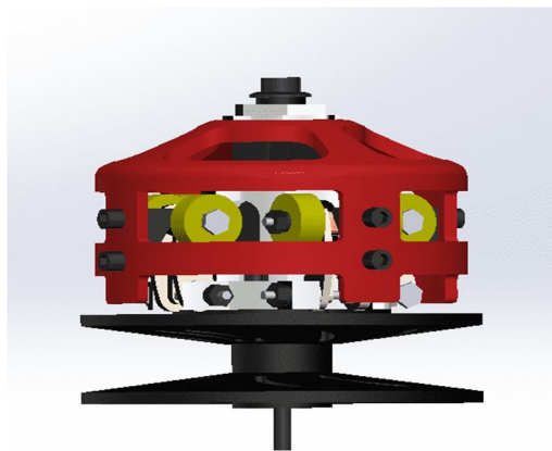
Fig 3.5 Expansion of the pulley in idle
