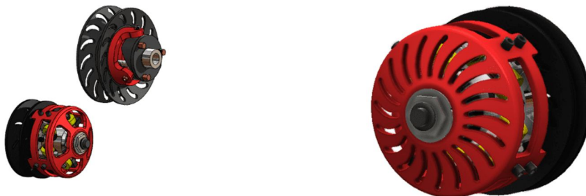
Fig 3.1 The assembly of CVT
