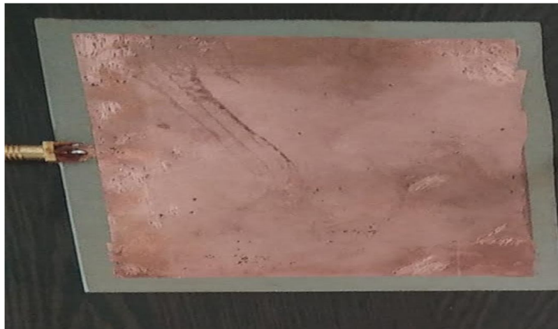
Fig. 7 Antenna built using RT-Duroid 6006 material
