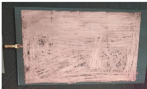
Fig. 4 Antenna built using RT-Duroid 5880 material
