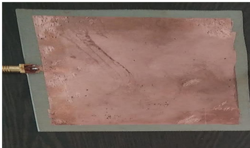
Fig. 7 Antenna built using RT-Duroid 6006 material
