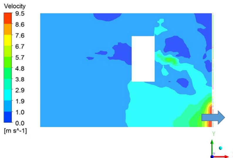
Figure 7: FDS velocity distribution at middle of height
