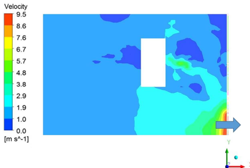
Figure 7: FDS velocity distribution at middle of height
