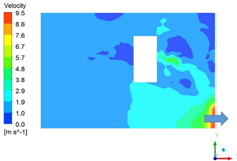
Figure 7: FDS velocity distribution at middle of height
