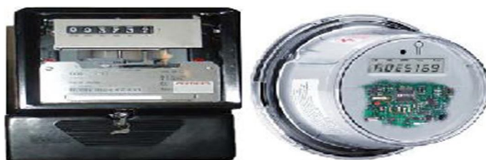
Figure 2.1: Traditional Electromechanical Meter Vs Electronic meter [9]
