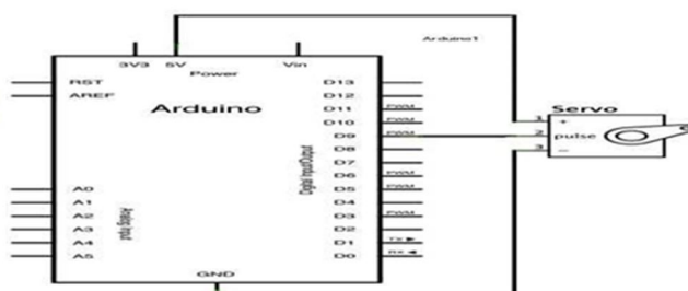
Fig 7. Schematic diagram of servo motor connection with Arduino
