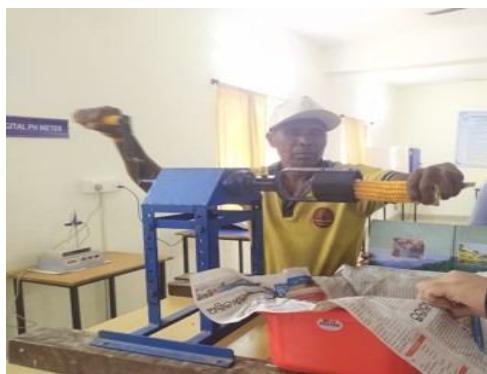
Fig.10 manually shelling of maize by rotary maize sheller (male)
