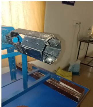
Fig.2 Rotatable octagonal hollow cylinder
