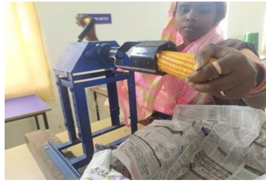
Fig.11 manually shelling of maize by rotary maize sheller (female)
