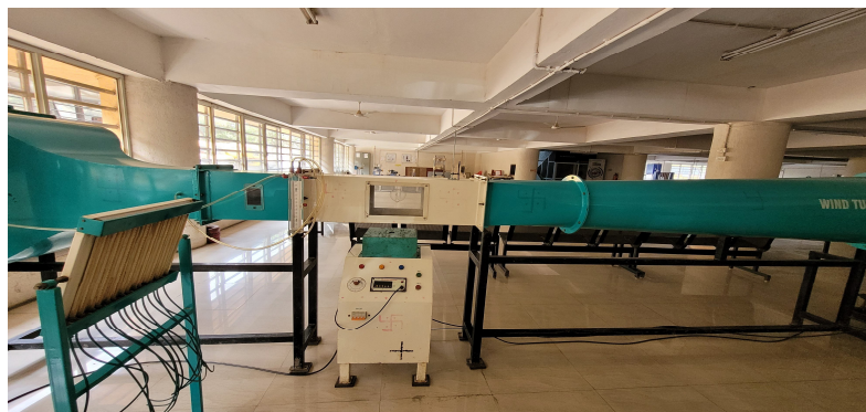
Fig. 5 Wind tunnel set-up (Test Section)
