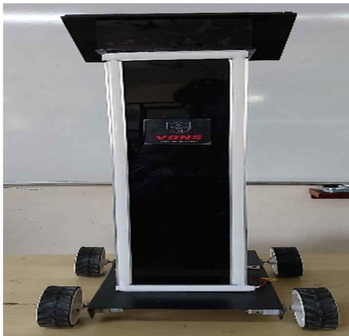
Figure 1: Line following Tour Guide AGV
