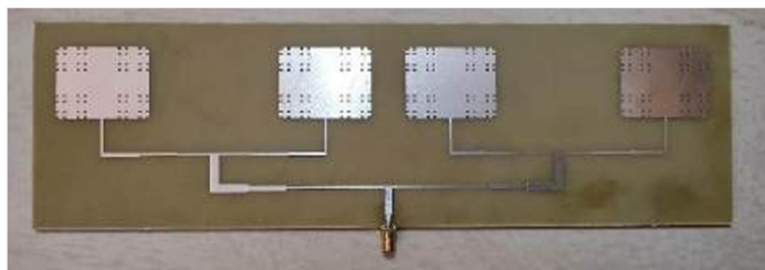
Figure 14:4 Element Fractal geometry Array Antenna
