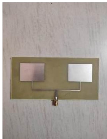
Figure 4: 2 Element Array Antenna
