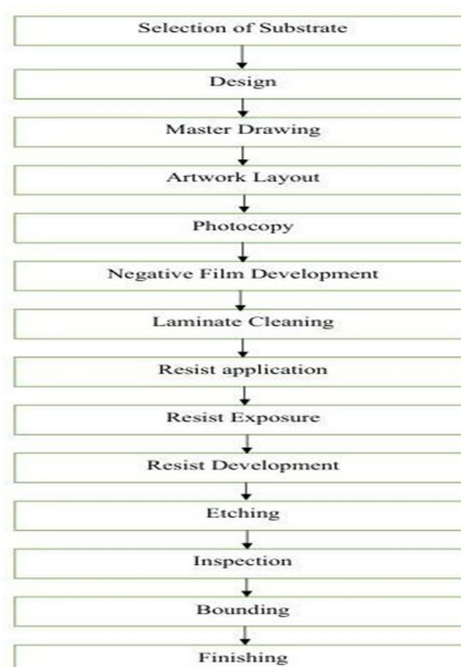
Figure 21 Flow chart of Fabrication process
