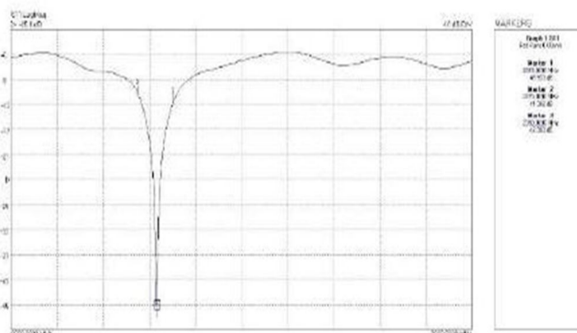
Figure 52 Practical Return loss vs Frequency of 8 element
