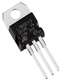
Fig.4: Voltage Regulator (LM 7805)
