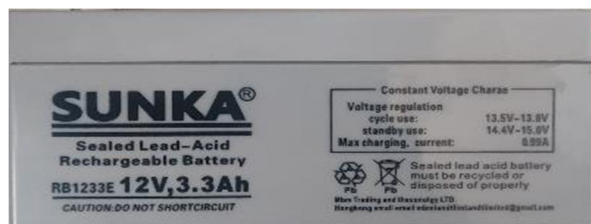
Fig 4.6: 12V, 3.3AH lead acid battery
