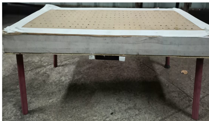
Figure1. Automated Air Conveyor
