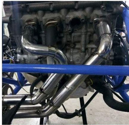
Fig 15 Exhaust runners manufactured
