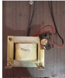
Fig : Step down transformer
