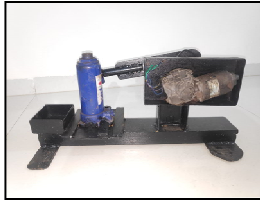
Fig 1. Motorized Hydraulic Jack system (1 st view and 2 nd view)
