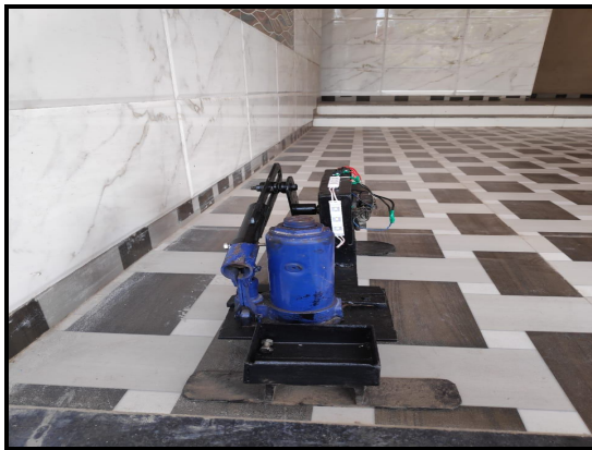
Fig 1. Motorized Hydraulic Jack system (3 rd view and 4 th view)
