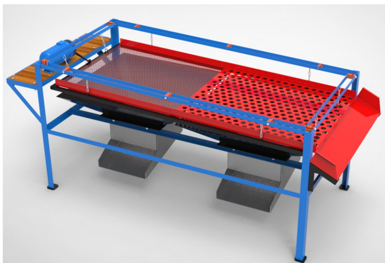
Figure 1 Design of Multi-Sieve Sand Sieving Machine
