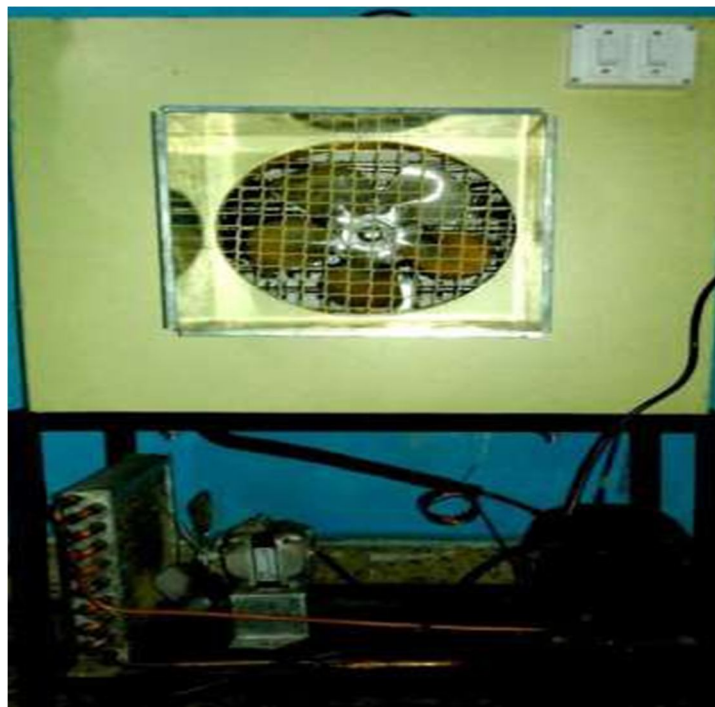
Fig. 4.3: VCRS based actual air cooler
