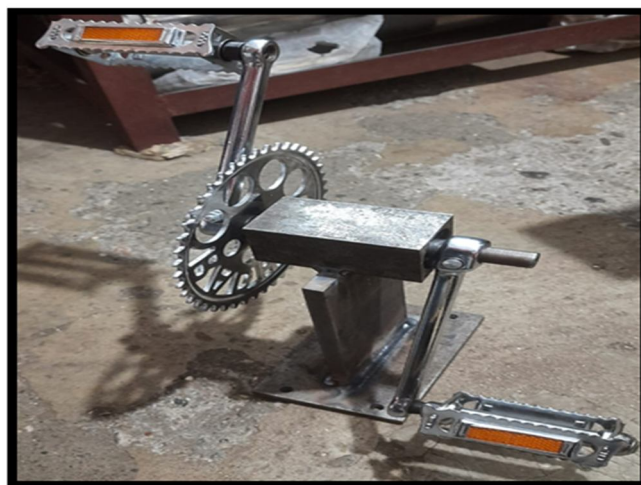
Fig 1 Lower housing with shaft and bigger sprocket
