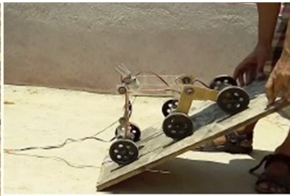
Fig 7 Photo image of on angle surface about 45° inclination
