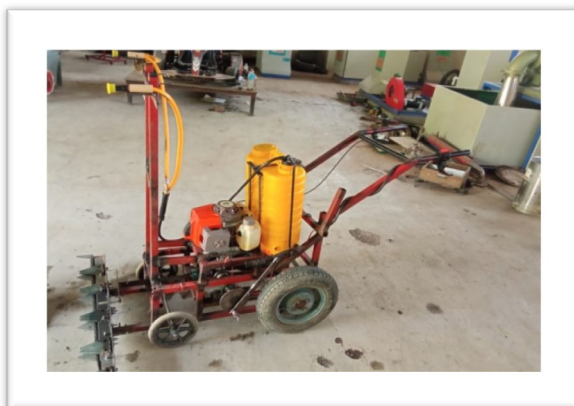
Figure 5: Working Model of Multi Nozzle Wheel Spray Pump
