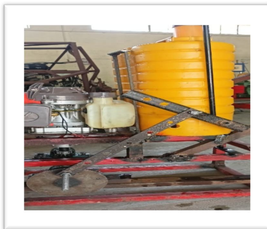
Figure 3: Assembly of Crank, Connecting Rod & Piston
