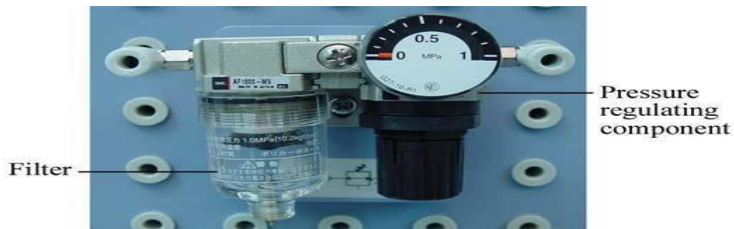
Fig: 3 Pressure regulating component
