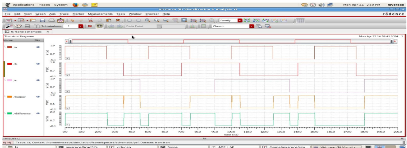
Fig.4 Output of 10T Full subtractor
