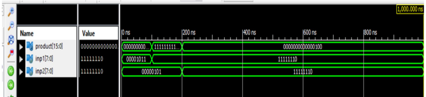
Fig. 8 Radix-8 Booth Multiplier simulation results.
