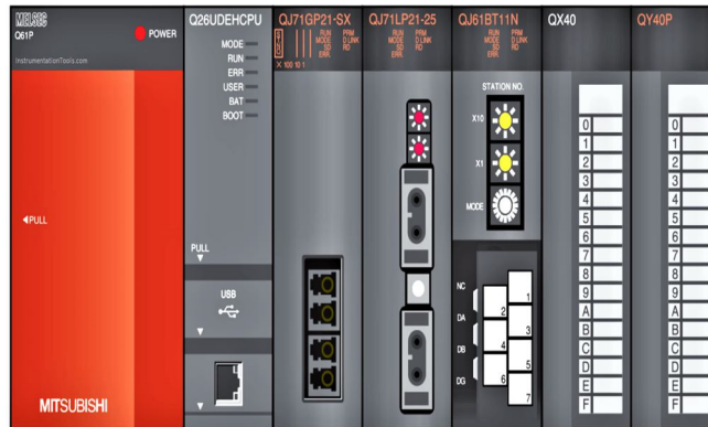
Fig. no: 2.2 Mitsubishi Q-SERIES PLC Controller.
