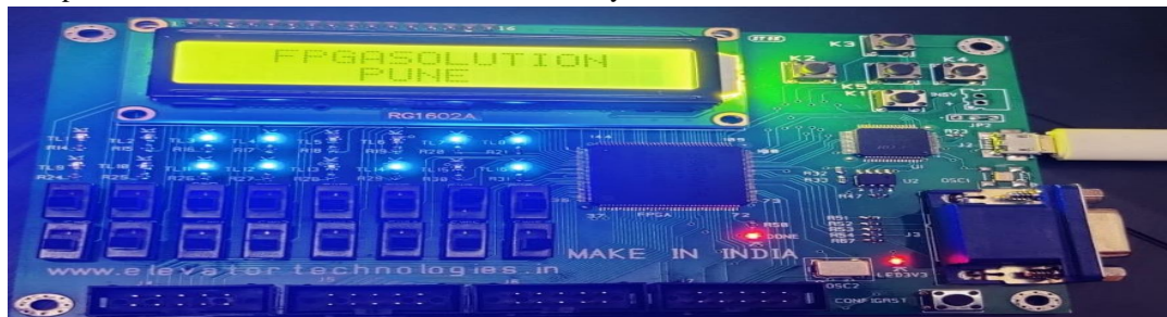
Fig. 9 : FPGA prototyping results of RISC MIPS processor
