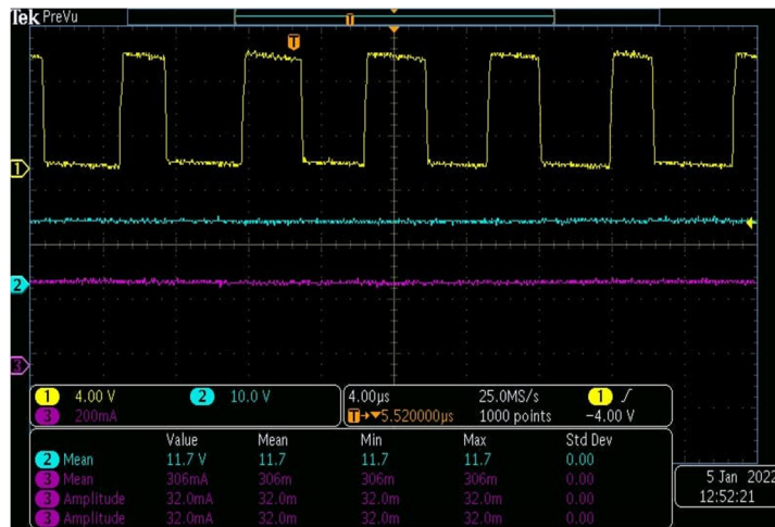
Figure 6: Hardware Input Waveforms: Yellow-Gate-source Voltage, Blue-Input Voltage Purple-Input Current
