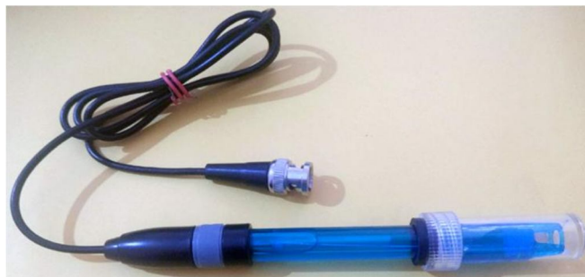
Fig. 3 Gravity PH Sensor.
