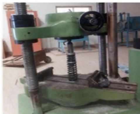
Fig 7.1: Test conducted on UTM of shock absorbers
