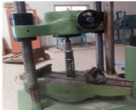
Fig 7.1: Test conducted on UTM of shock absorbers
