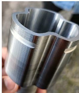
Fig. 7 VMC Machined CV profile
