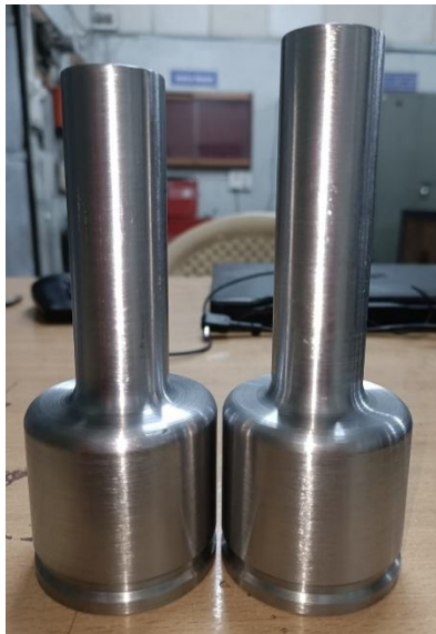
Fig. 4 Geometry after lathe machining
