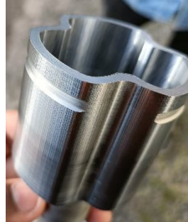
Fig. 7 VMC Machined CV profile
