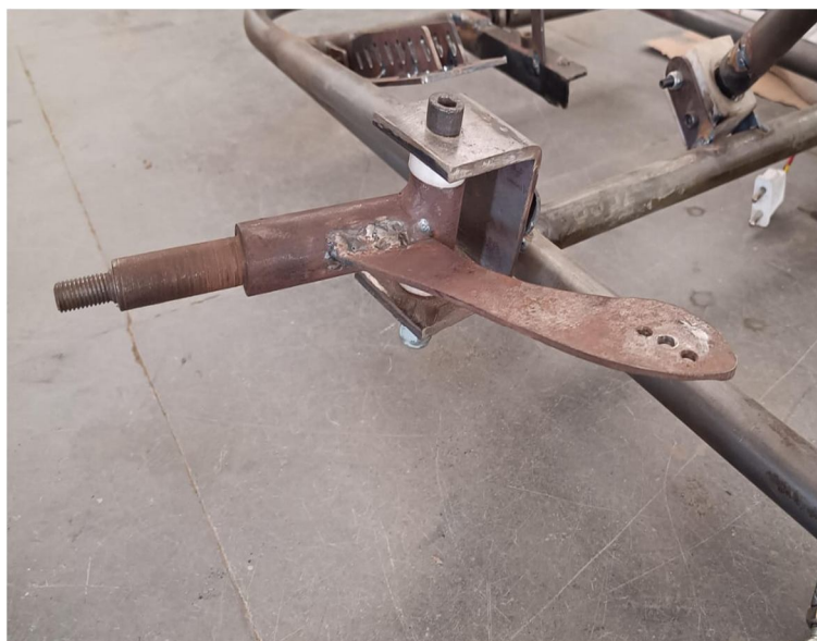
Fig 5.2(ii): Model of Knuckle
