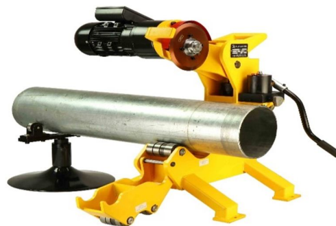
Fig: 7.1: Cutting of tubes.
