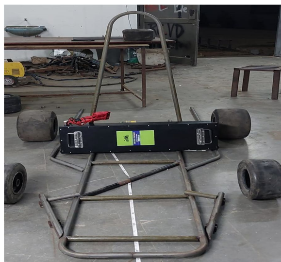
Fig: 7.1.4(ii): Welded Chassis
