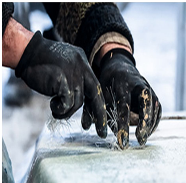
Fig 7.2(i): Fibre glass layup
