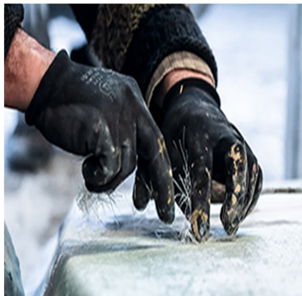
Fig 7.2(i): Fibre glass layup
