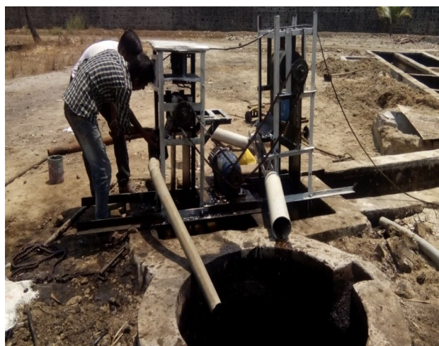
Fig.9. Modifying Oil Skimmer Machine
