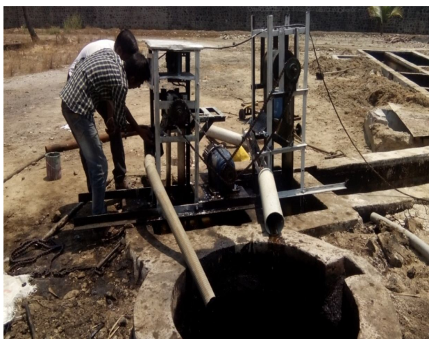
Fig.9. Modifying Oil Skimmer Machine
