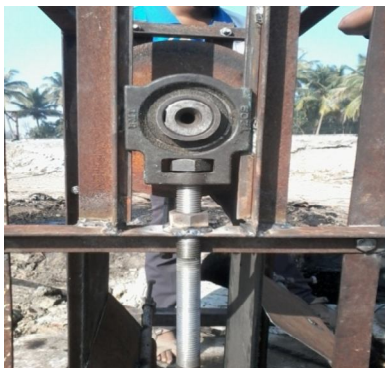
Fig.7. Sub-assembly of tightening arrangement
