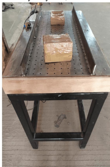
Fig : 5 : Actual Air Conveyor With Conveying Products
