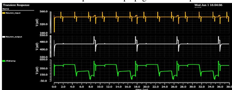
Fig 8. Transient response of the spike generator circuit
