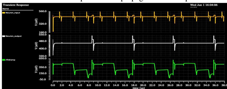
Fig 8. Transient response of the spike generator circuit
