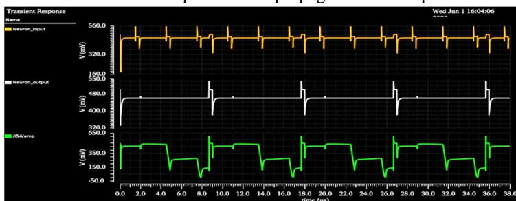
Fig 8. Transient response of the spike generator circuit
