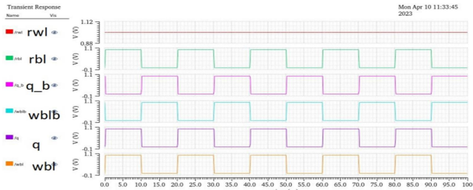
Figure 4.8: 8T read operation output waveform
