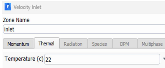
Figure Boundary Conditions Initial velocity & Air Temperature
