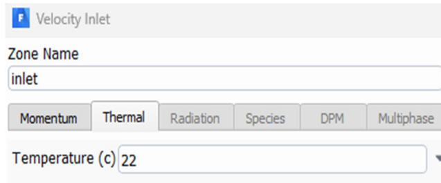
Figure Boundary Conditions Initial velocity & Air Temperature
