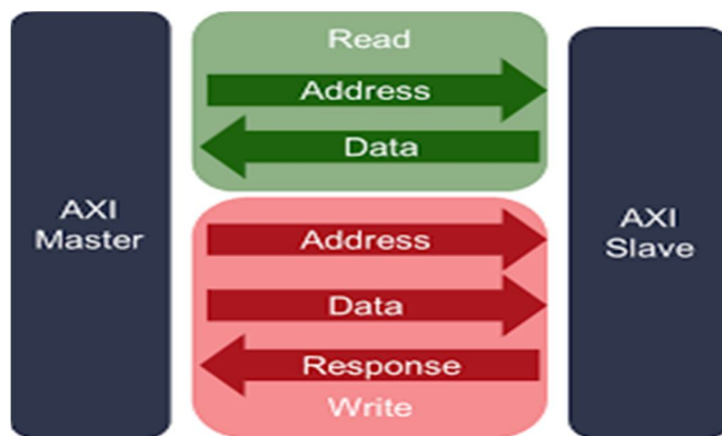
Fig. 3 Architecture of AXI
