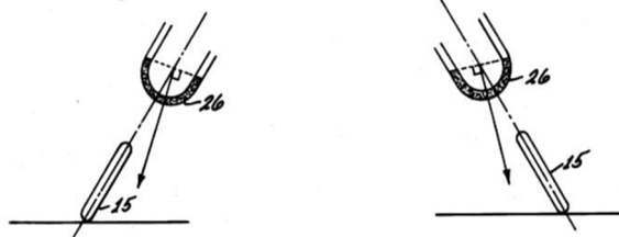
Fig. 13 Various Position at which guidable cornering light gets activated
