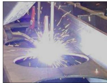
Fig4. Fabrication Process: Welding The Separated Tee-Sections Together
