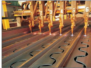
Fig3. Fabrication Process: Flame Cutting Of Hot-Rolled Profiles
