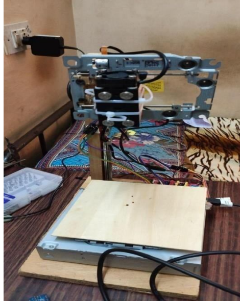
Fig.8: CNC based laser engraver Hardware module
