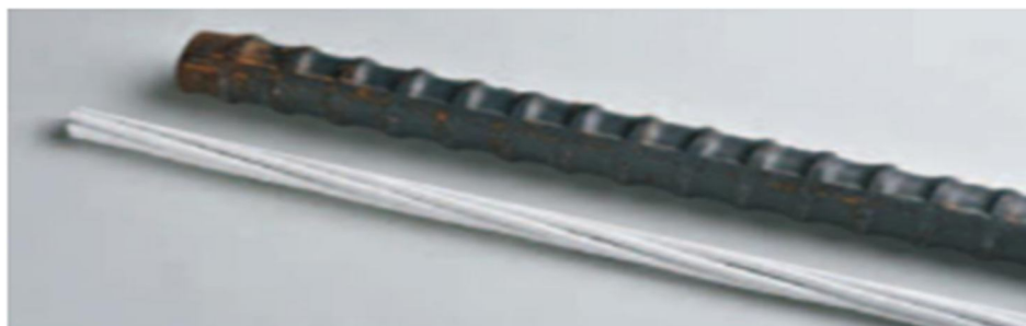
Size Comparison of Strand Rods Vs Rebar
