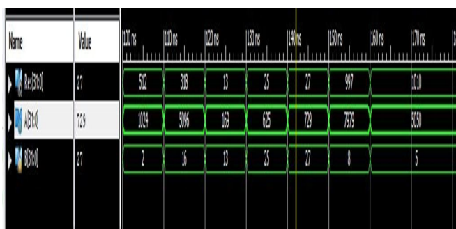
Fig : Output waveform of Divider.
