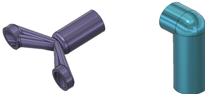
Figure 20: On left: Connector Pipe for Receiving Tank; On Right: For Skimming Tank.
