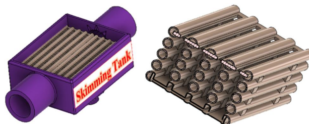
Figure 9: On left: Isometric View; On Right: Hollow Cross sectional View of the Oil Filter w/ Skimming Tank
