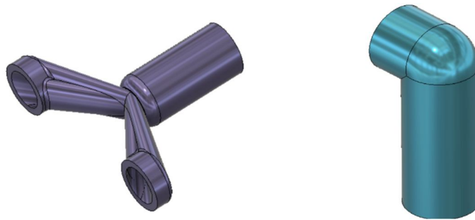
Figure 20: On left: Connector Pipe for Receiving Tank; On Right: For Skimming Tank.
