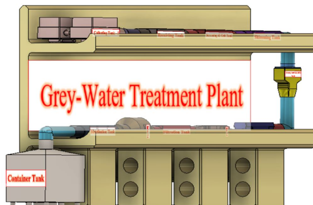
Figure 22: Front View of Grey Water Treatment Plant.
