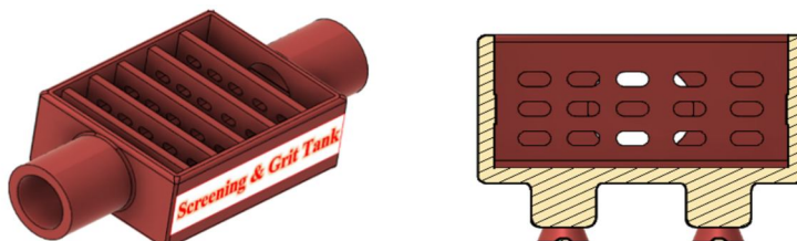
Figure 8: On left: Isometric View; On Right: Cross sectional Front View of the
