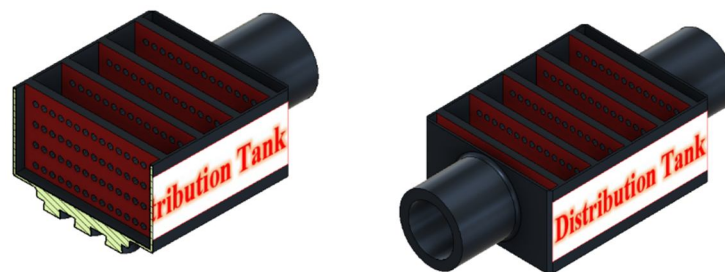
Figure 19: On left: Isometric View; On Right: Cross sectional View of the Distribution Tank w/ Section planes
