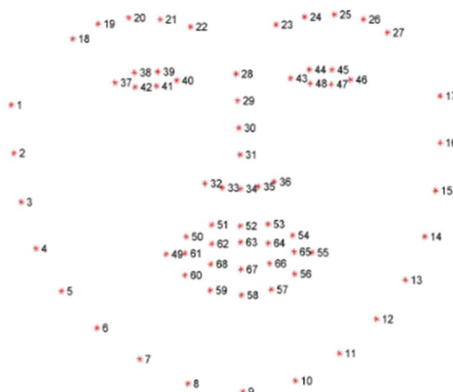
Figure 2: Sagonas C., Zafeiriou S., (n.d.). The 68-points mark-up used for annotations.
