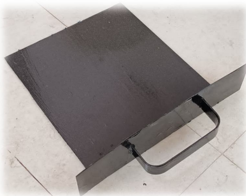
Fig. 8 Scrap inserting and removing plate
