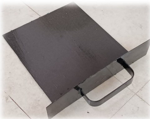
Fig. 8 Scrap inserting and removing plate
