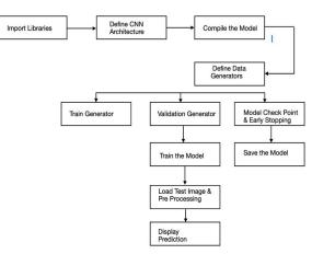
The flow diagram for Fake notes prediction system would typically include image analyzer image enhancement, image segmentation, feature extraction, classifier and detection. The datasets contain the images classified in different folders and these folders are used accordingly to train the CNN.
