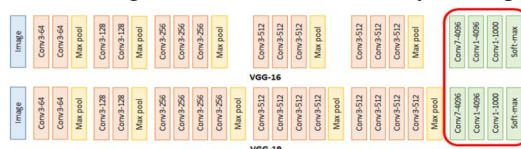
Fig. 3. Architecture of VGG16 and VGG19
