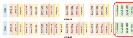
Fig. 3. Architecture of VGG16 and VGG19
