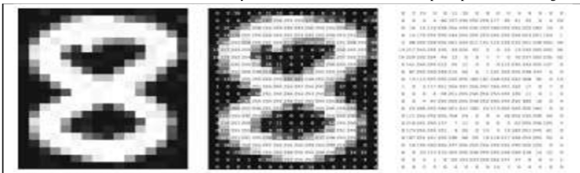
Fig.3 A computer sees an image as an array of numbers (34)
